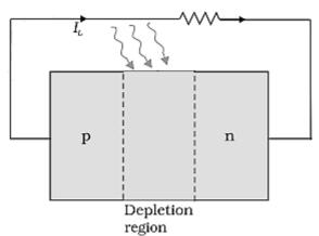
The generation of emf by a solar cell, when light falls on, it is due to the following three basic processes: generation, separation and collection—
