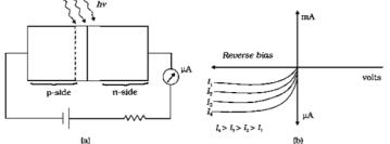
It is easier to observe the change in the current with the change in the light intensity if a reverse bias is applied. Thus photodiode can be used as a photodetector to detect optical signals.
